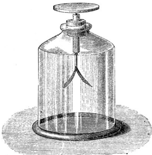
Figure 2-2. Gold leaf electroscope. From Silvanus P. Thompson, Elementary Lessons in Electricity & Magnetism (New York: Macmillan, 1901), 16.
